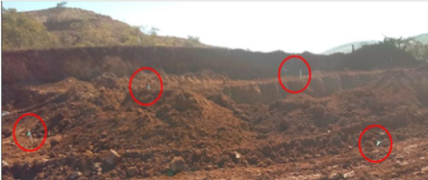
Figure 1. The mine relied on physical stakes to identify ore and dig boundaries, which were difficult to see.
