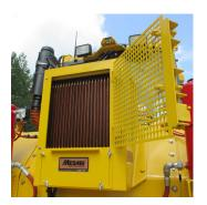
**Relocated Hydraulic Cooler**
