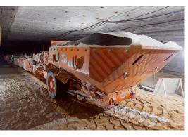
The FCT is a product of Komatsu's commitment to enabling customers to consistently produce at the lowest cost per ton over the life cycle of the equipment. Not only does the life cycle cost per ton of the FCT itself compare favorably to other forms of haulage, the increased production and efficiencies that it unlocks in the typical continuous miner section improve the cost per ton performance of the entire operation.
