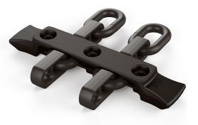
Broadband chain now comes with an innovative 'S' shaped center post on the vertical link which is designed to prevent knuckling of the chain and therefore reduce the likelihood of chain wreck events.
