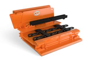
Komatsu manufactures all the key elements for the armored face conveyor (AFC) including the head and tail frames, linepans, gearboxes, sprockets, couplings and shearer haulage systems. The design of the Joy AFC uses cast steel sigma sections with exacting tolerances. This casting technology eliminates the weld fabrication of less reliable clevis and pan connections. The cast design
