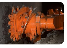
To meet your unique conditions, we custom-design your drums and manufacture them using our own patented design three-axis digital lacing machine to achieve precise bit locations and angles. The bit positions for each drum are digitally recorded for traceability. Final machining of drum bores is accomplished with state-of-the art CNC turning centers to achieve a precise fit for your Joy shearer.
