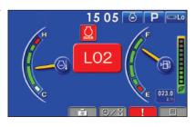
displayed, a caution lamp blinks and a warning buzzer sounds to alert the operator to take action.
