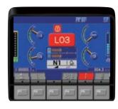
addition, countermeasures are indicated in four levels to help prevent major machine issues. Replacement times for required planned maintenance services are also indicated.
