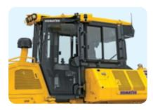
vibration for the operator and discourage dust from entering the cab. In addition, side visibility is increased because external ROPS (ISO 3471) structure and posts are not required.
