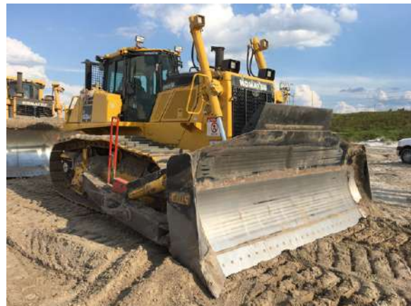
Semi-u blade dual tilt and pitch abrasion resistant spec
