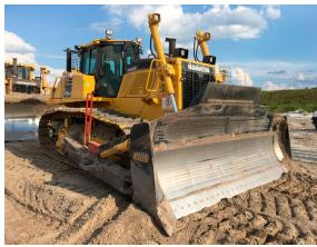
Semi-u blade dual tilt and pitch abrasion resistant spec
