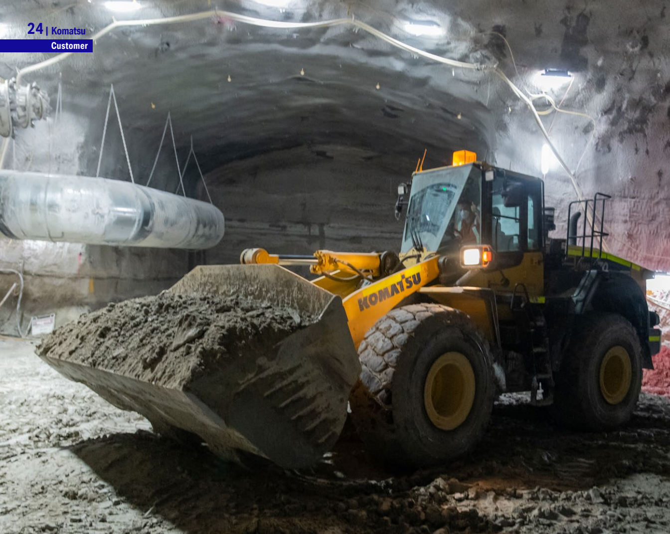
Pictured above: One of the three Komatsu WA470-7 wheel loaders fitted with a 4.65 cu m bucket, used for underground applications.
