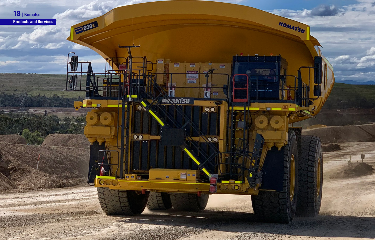
Pictured: This Komatsu 930E-5 haul truck is the first Tier 4 Final version of this unit in Australia.
