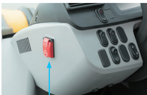
Engine shut down secondary switch
