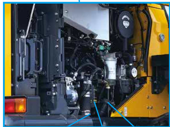
Engine oil dipstick Fuel filter Engine oil fill
