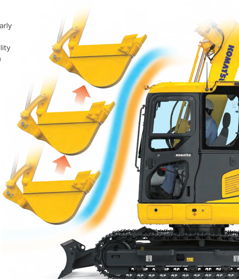
Interference avoidance area Automatic stop area
