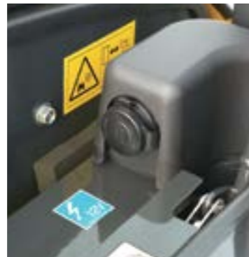
12V external power outlet This power source outlet is a cigarette lighter socket which is the same as that of automobile.
