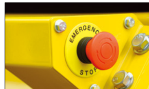
E-Stops Allow compliance to site safety requirements.
