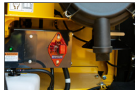
Battery Isolation Single pole, lockable Bosch-type battery isolation.
