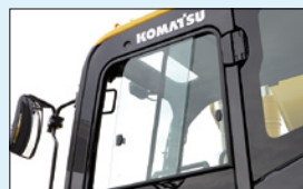
Remote intermittent wiper with windshield washer
