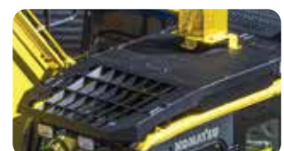
Bolt-on Top Guard OPG level 2 (ISO 10262) for falling object protection.
