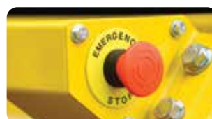
E-Stops Allow compliance to site safety requirements.
