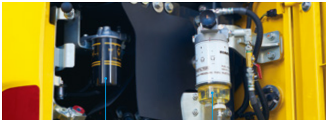
High efficiency fuel filter
