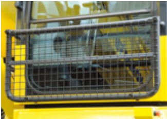
Lower Front Window Guard Protects cabin windscreen against rocks and debris.
