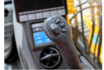
Proportional Hand Controls Enables proportional hand control of attachment speed
