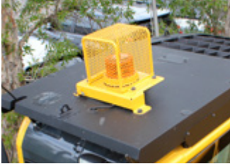
Rotating Amber Beacon Fitted with factory guard.
