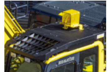
Bolt-on Top Guard OPG level 2 (ISO 10262) for falling object protection.
