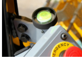
Level Indicator, Overload Alarm & Anti-Burst Valves Enable safety and compliance when lifting suspended loads
