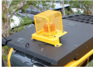
Rotating Amber Beacon Fitted with factory guard.
