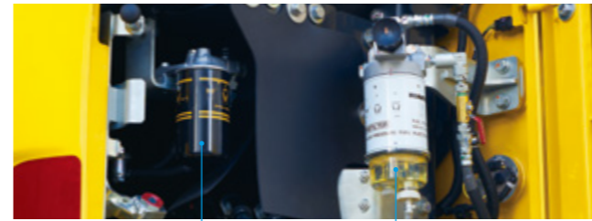
High efficiency fuel filter Fuel pre-filter (With water separator)
