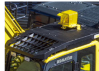
Bolt-on Top Guard OPG level 2 (ISO 10262) for falling object protection.
