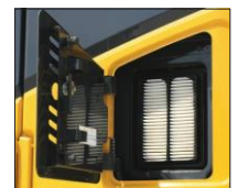
External air conditioner filter
