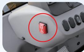
Secondary engine shutdown switch
