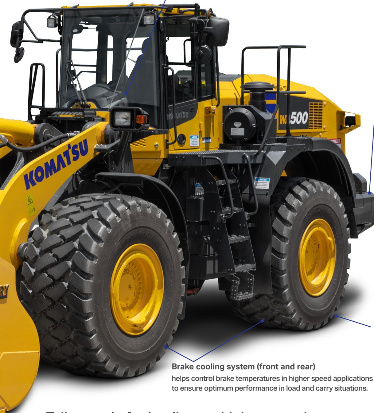
**875/65 tires** increase ground contact area for improved stability. The low profile also reduces sidewall flex for more stability while dumping into trucks or hoppers.
