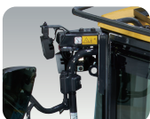
Anchor point of tie-off
