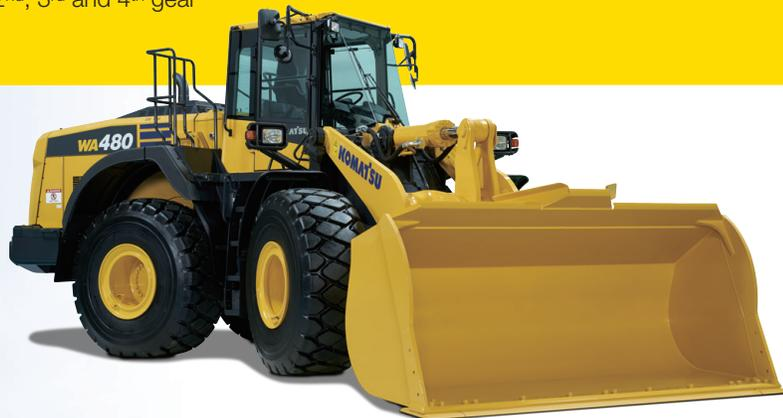
The **Yard Loader arrangement** features a 7.2 yd<sup>3</sup> genuine Komatsu high performance bucket, low profile 775/65/ R29 tires, an improved brake cooling system and a heavier Yard Loader counter weight, and is designed to three pass typical on-highway trucks.
