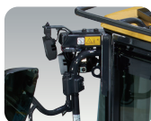
Anchor point of tie-off
