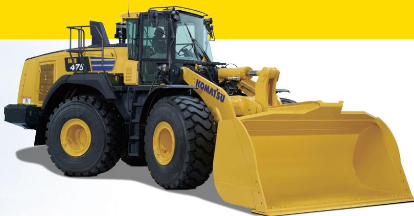
A powerful **Komatsu SAA6D125E-7 engine** provides a net output of 216 kW **290 HP** with 17% improved fuel consumption. This engine is EPA Tier 4 Final emissions certified.
