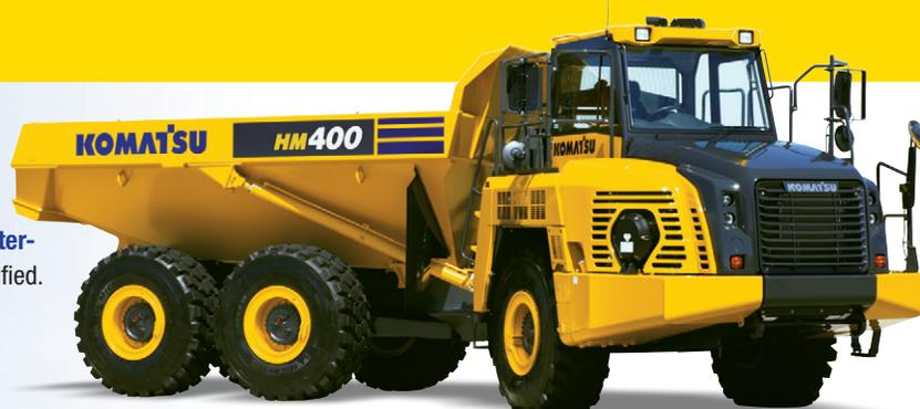
**Komatsu SAA6D140E-7 variable geometry turbocharged and after-cooled 15.24 liter diesel engine** is EPA Tier 4 Final emissions certified.
