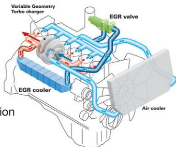
**Variable Geometry Turbocharger (VGT) system**
