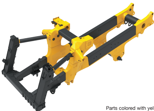
Parts colored with yellow show cast-steel components.
