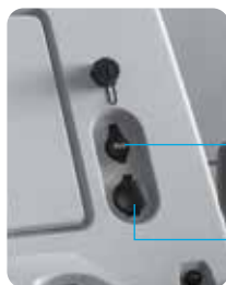
Cigarette lighter (DC12 V) AUX terminal DC12 V electrical outlet
