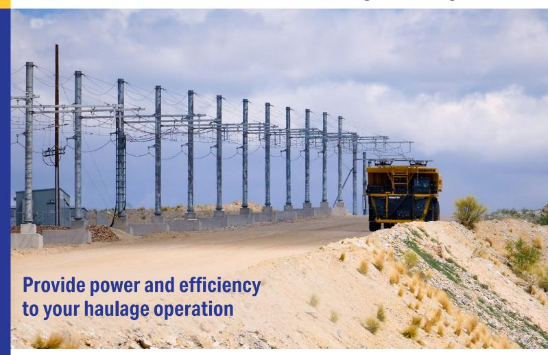
We understand uphill haulage operations can increase fuel consumption and physically overwhelm your haul trucks. Komatsu offers its trolley assist system to provide the power and efficiency your operation needs to help reduce fuel costs, lessen the strain on your vehicles and optimize your mining business.
