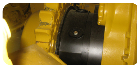
Final drive seal guards Provides an extra level of protection from wear and contamination due to debris. The clamshell design ensures a tight fit around the final drive housing, used hardened hardware and bolt head protectors.
