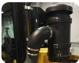
Cab air precleaner Removes large particles and extends the life of the cab air filter.
