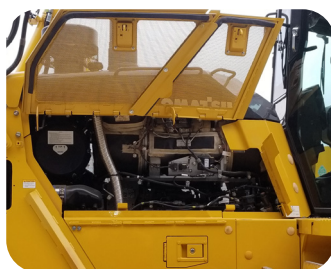
Additional sealing and deflector bars Chassis and door seals reduce amount of debris entering engine compartment. Deflector bars redirect larger debris.
