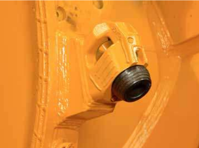
The sleeve can be readily extracted by removing the protective cap on top of the block and attaching a hydraulic supply.
