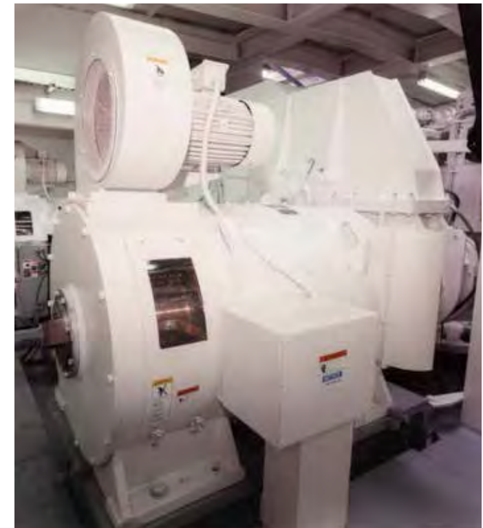
Figure 39 Typical hoist motor with a centrifugal type blower
