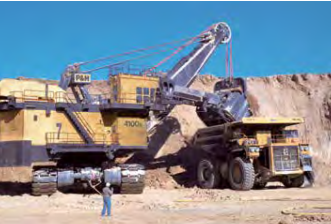
Figure 20 A shovel’s work cycle consists of digging, swinging, dumping, and returning to the bank.
