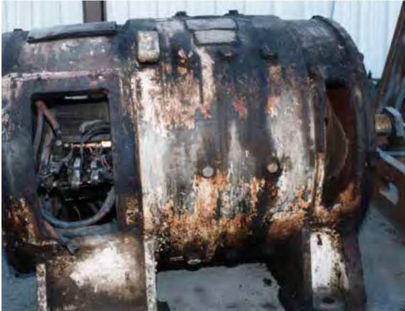
Figure 64 Improper maintenance, abuse or other detrimental conditions can lead to catastrophic motor failure.
