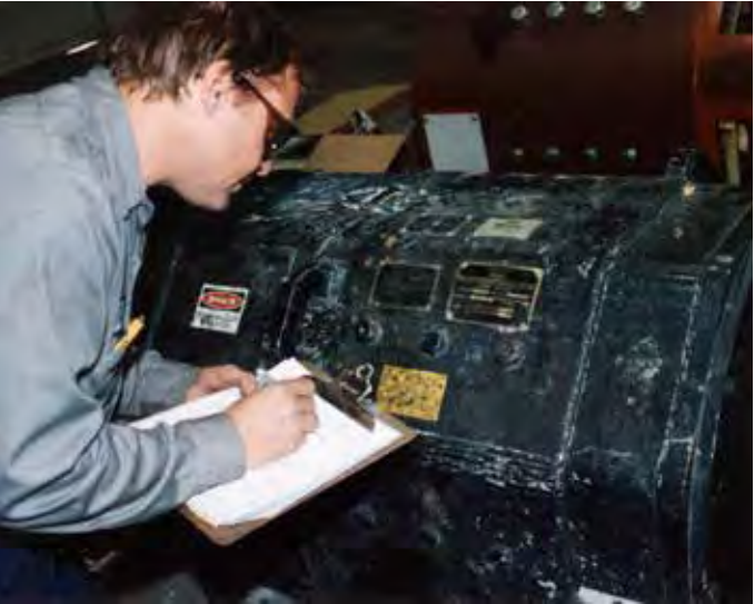
Figure 71 Motors are steam cleaned and inspected upon arrival at a Komatsu rebuild center.
