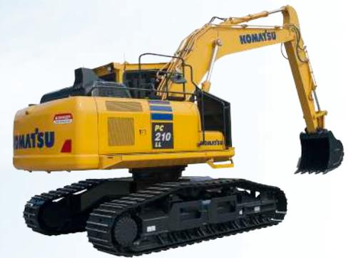
**Grip strut walkways and handrails** located on the machine upper structure provide a more convenient work area along both sides of the machine for maintenance and service.
