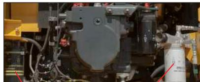
Fuel filter      Fuel pre-filter (with water separator)
