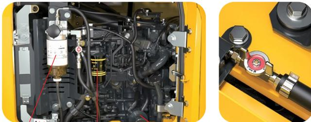
Fuel pre-filter (With water separator) High efficiency fuel filter
