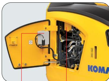
Washer tank Auxiliary hydraulic circuit return filter
