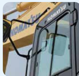
Remote intermittent wiper with windshield washer
