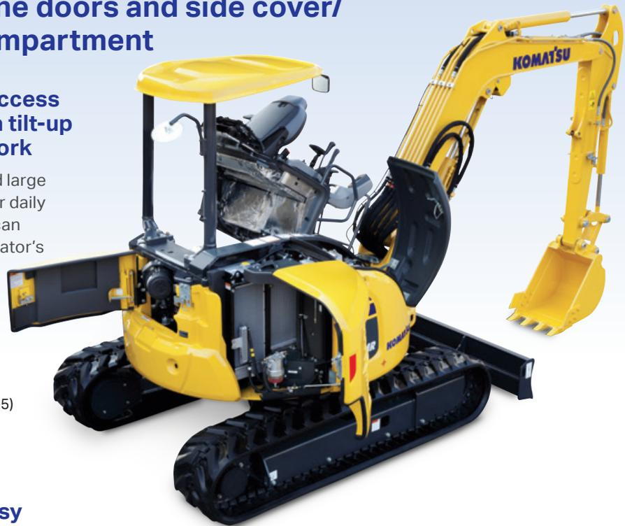
Tilt-up floor mechanism and full-open cover for the canopy model (PC45MR-5)
