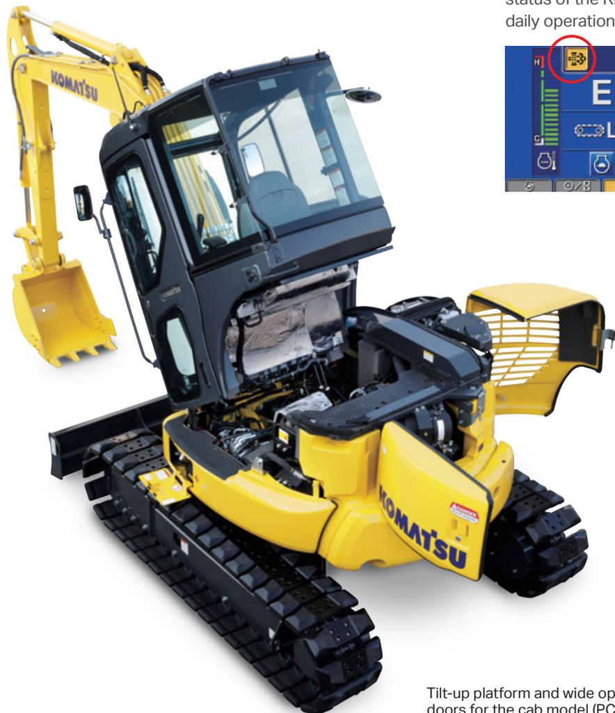
Tilt-up platform and wide opening doors for the cab model (PC55MR-5)
