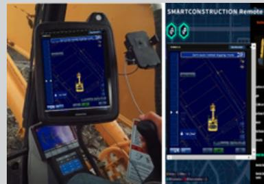
View or navigate machine monitor live with operator.
