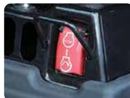
Secondary engine shutdown switch at base of seat to shutdown the engine.
