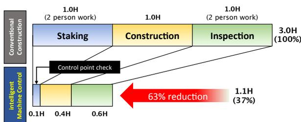
\* When used by a qualified iMC operator, the Komatsu intelligent Machine Control system increases construction efficiency.
