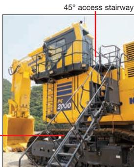
45° access hydraulically operated stairway
