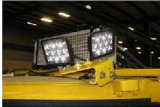
The two hood-mounted lights are replaced with four guarded LED work lights mounted on the lift cylinders, shining light in front of the trash rack.
