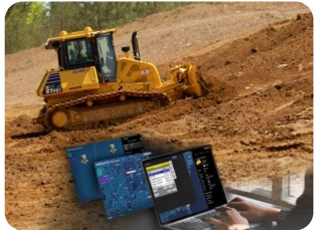
An IMC dozer is capable of dozing to plan with incredible precision and efficiency when working off a 3D design.
