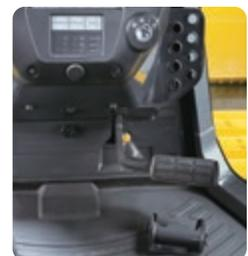
**Decelerator mode:** The pedal modulates engine rpms and vehicle travel speed. It can be used for all applications.
