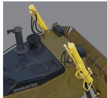
**Factory Installed Machine Control System For Quality, Durability**
