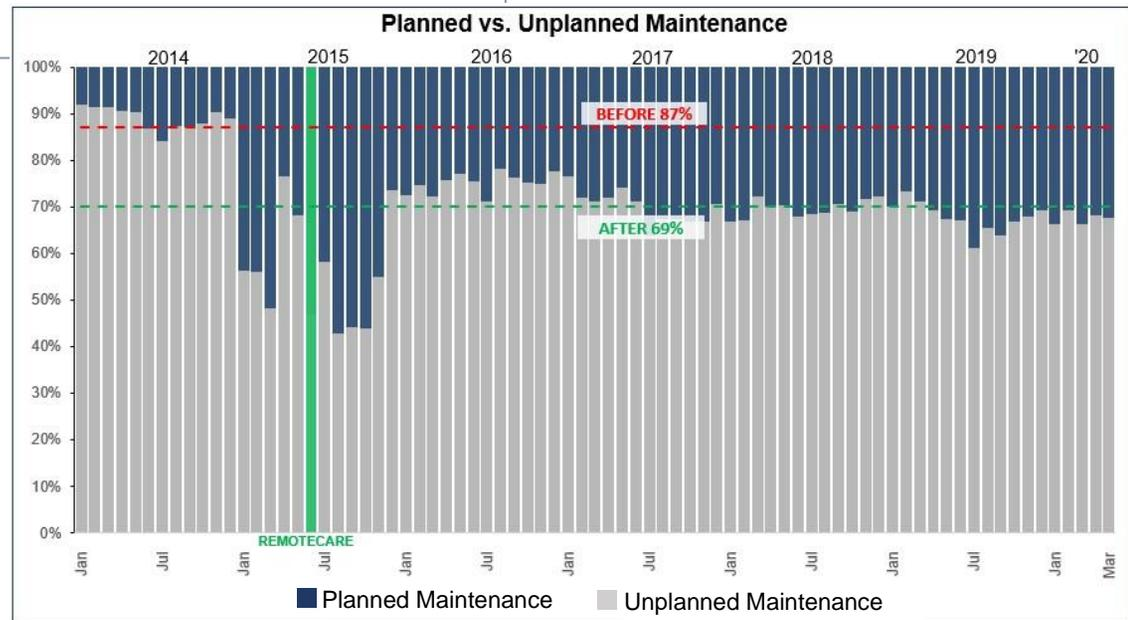
Figure 2. Unscheduled maintenance decreased by nearly 21% after implementing the MineCare system and RemoteCare service
