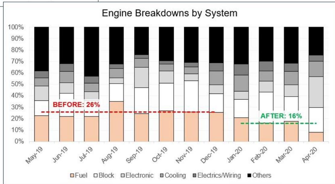
Figure 8. The percentage of engine breakdowns as a result of fuel system failures has declined by 38%.
