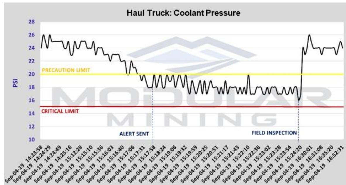
Figure 3. The RemoteCare analyst leveraged data from the MineCare system to generate a report for the site's maintenance technicians, which identified a drop in the engine's coolant pressure below the allowable and configurable threshold.
