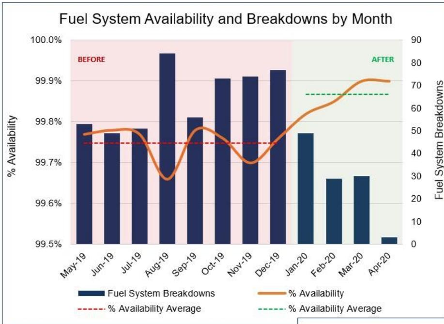
Figure 7. The new fuel system monitoring parameters helped the mine increase its fuel system availability, correlative to a decline in system breakdowns
