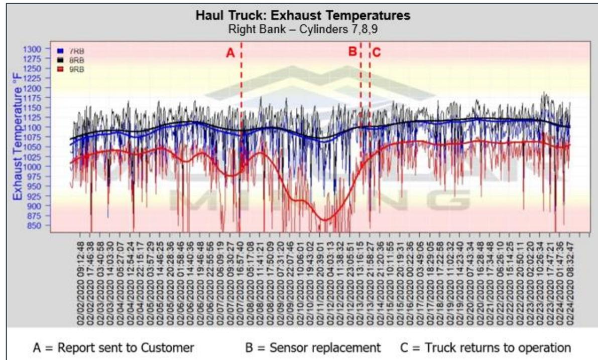
Figure 5. After the faulty sensor was replaced, the truck was returned to operation and exhaust temperatures recovered.
