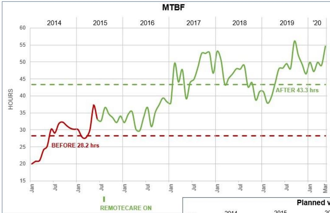
Figure 1. The mine's mean time between failure (MTBF) increased by more than 15 hours (53%) after implementing the MineCare system and RemoteCare service
