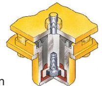
The large ROPS/FOPS cab is mounted with Komatsu's unique viscous mounts. The low-noise engine, hydraulically-driven fan, and hydraulic pumps are mounted with rubber cushions, and the cab sealing is improved to provide a quiet, low-vibration, comfortable operating environment.
