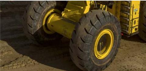
Komatsu pressurized axle housings enhance reliability by maintaining an air-cooled, dust-free environment for the traction motors and disc service brakes.
