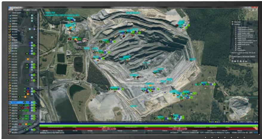
**Utilization** presents an overview of the machine idle time by location and machine. More detailed data is provided on the Idling Insights and Summary tabs.
