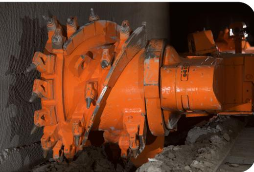
*To meet your unique conditions, we custom-design your drums and manufacture them using our own patented design three-axis digital lacing machine to achieve precise bit locations and angles. The bit positions for each drum are digitally recorded for traceability. Final machining of drum bores is accomplished with state-of-the-art CNC turning centers to achieve a precise fit for your Joy shearer.*
