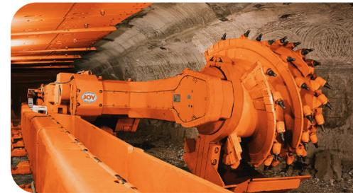
*Industrial minerals mining is growing, and we offer complete longwall solutions designed specifically for salt, potash, gypsum and trona. Fully mechanizing the extraction of industrial minerals can improve safety while increasing productivity. Customers utilizing these advancements have seen up to 40% cost savings versus the traditional drill-and-blast method.*
