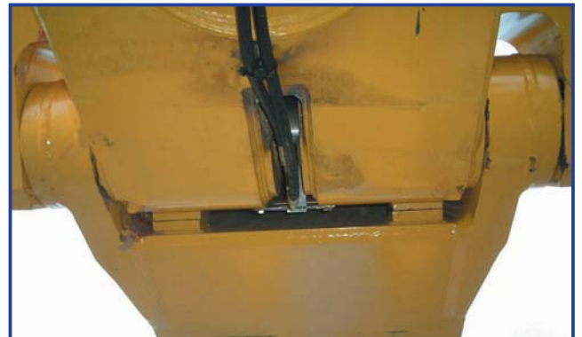
Insertion & Removal of Pin by Hydraulic Cylinder
